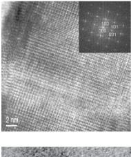
**Fig. 2.** Nanowire of Fig. 1 in high-resolution mode Inset : Fourier transform. Reflections (d = 0.4434 nm 0.3342 nm and 0.4900 nm) are indexed as Fe<sub>3</sub>C 001, 101 and 100, respectively
