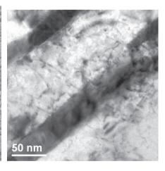
**Fig. 3.** Same as Fig. 2 for cross section of a cementite nanowire piercing the image plane
